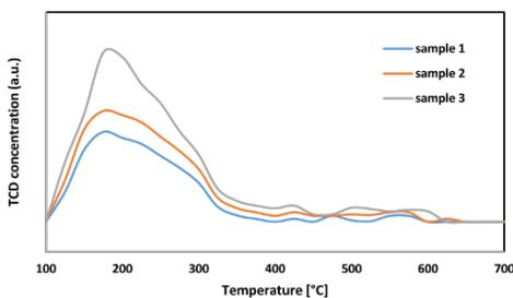
The binding energy of the adsorbate phase can be determined by means of a TPD measurement. A material previously loaded with adsorbate is heated under defined conditions, which leads to desorption of the previously adsorbed molecules. The desorption is detected by downstream analytics (TCD or MS).
