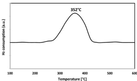
TPR is used to investigate the reducibility or thermal behavior of catalysts as a function of temperature. Usually H<sub>2</sub> is used as reductant. The figure shows the TPR data measured for a nickel oxide sample (NiO), according to:
