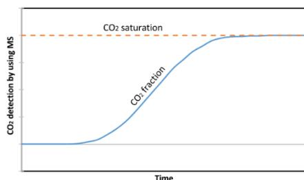
The measurement of breakthrough curves is a commonly used method for the evaluation of adsorption capacity and corresponding kinetics: A gas mixture (e.g. CO<sub>2</sub>-N<sub>2</sub>) flows through an adsorber filled with the sorbent. First, the preferred adsorbing component will be adhered by the material. After saturation, the component breaks through and is detected by suitable gas analysis.
